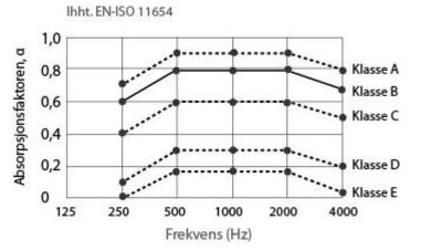
The above shows sound classes in relation to the absorption coefficient.
